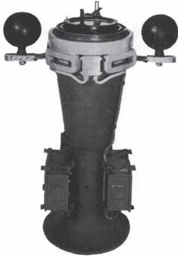
Figure 817. Type K degaussing compensation installation.
