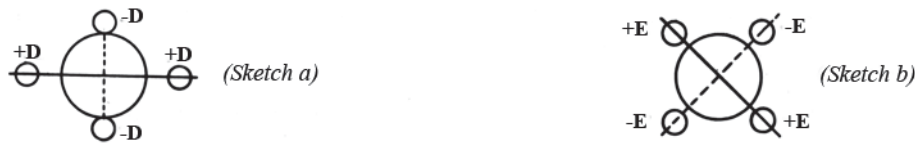
Figure 807. Summary of compass errors and adjustments.
