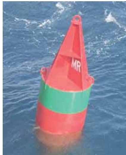
Figure 733a. Preferred channel or "junction" buoy.
