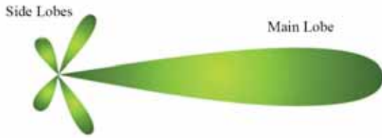
Figure 2306a. Freespace radiation pattern.
