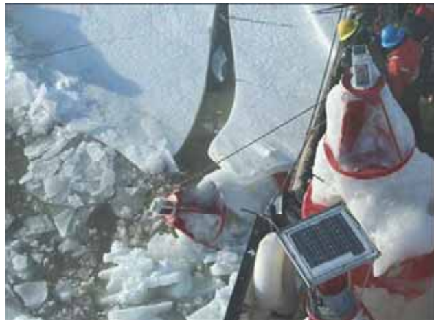
Figure 706. USCG recovering ice damaged buoys.
