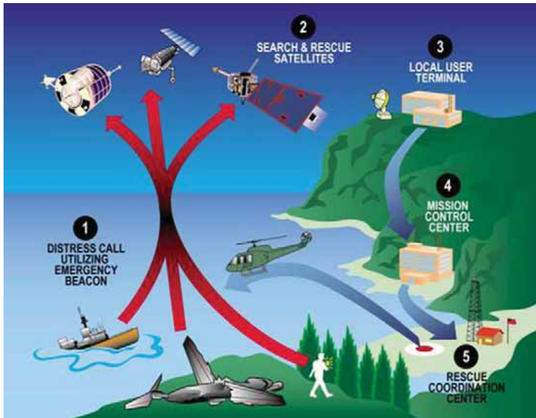
Figure 3016a. COSPAS-SARSAT System Overview. (1) Emergency locator transmitters (ELTs), EPIRBs, and personal locator beacons (PLBs) operate on the 406 MHz frequency. Each 406 MHz beacon transmits a unique digital code that identifies the type of beacon and that allows registration data to be associated with the beacon. The registration data provides information such as the beacon owner; the type of platform the beacon is associated with; emergency points of contact; and much more. (2) After the satellite receives a beacon signal, it relays the signal to ground stations referred to as local user terminals (LUTs). There are two types of LUTs: Low-Earth Orbiting LUTs (LEOLUTs) which receive and process alert data from the polar-orbiting satellites; and Geostationary LUTs (GEOLUTs) which receive and process alert data from geostationary satellites. (3) The LUT processes the data and transmits an alert message to its respective Mission Control Center (MCC) via a data communication network. (4) The MCC performs matching and merging of alert messages with other received messages, geographically sorts the data, and transmits a distress message to another MCC, an appropriate SAR authority such as a national Rescue Coordination Center (RCC) or a foreign SAR Point of Contact (SPOC). (5) The RCC investigates the beacon alert and launches assets to find the parties in distress when necessary.
