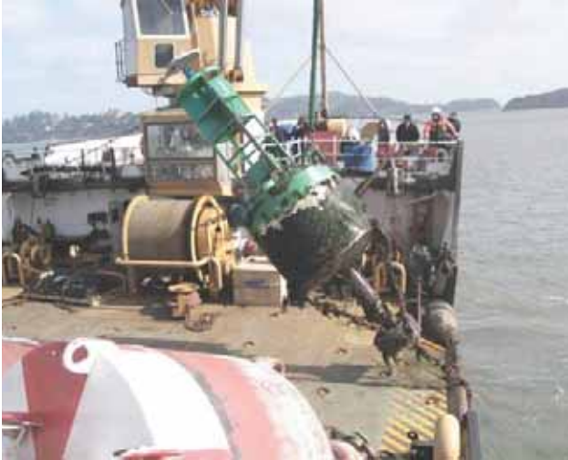
Figure 701a. Buoy with counterweight showing.
