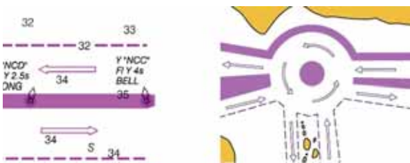
Figure 2904. Traffic separation scheme examples.
