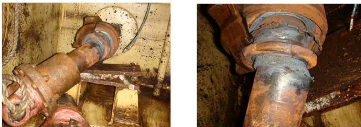
Figure 1 Destroyed shaft line at high speed due to whirling vibration
